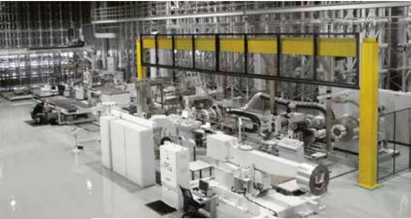
Machine protection lift gate XL for flexible and rapid plant access and optimum view of process
